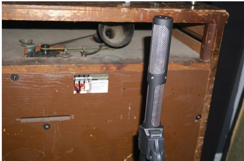
The Mesanovic Model 2S stereo ribbon microphone captures the sound of a Leslie cabinet during one of Russ Long's recent tracking sessions.
